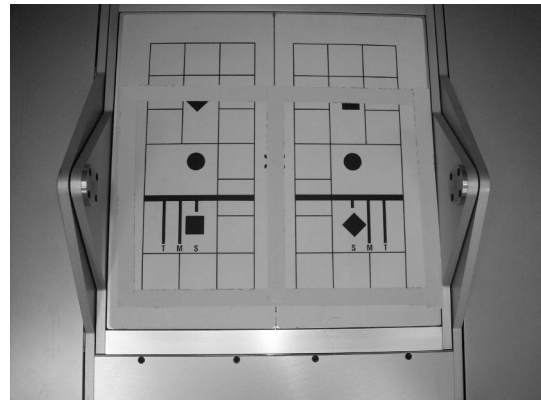
Figure 4. EquiTest® force plate with the dimensions of the Wii Fit Balance Board™ indicated by a tape outline.
